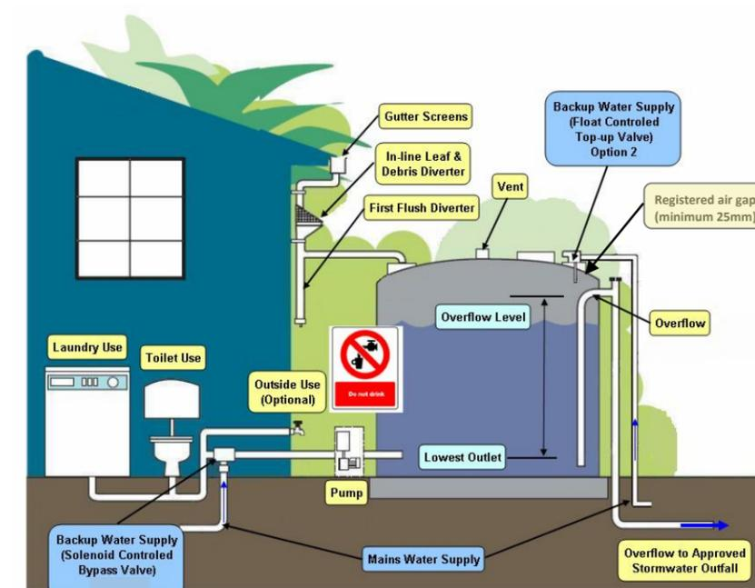
Figure 2: Rain Tank above ground - typical components
