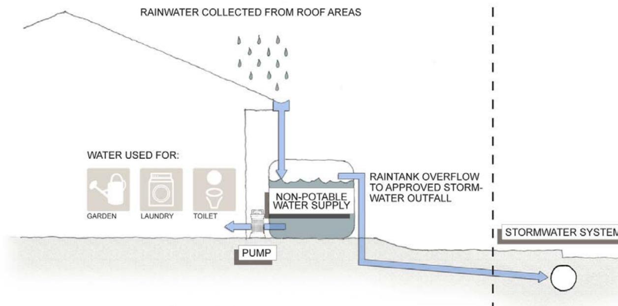
Figure 1: Typical arrangement
