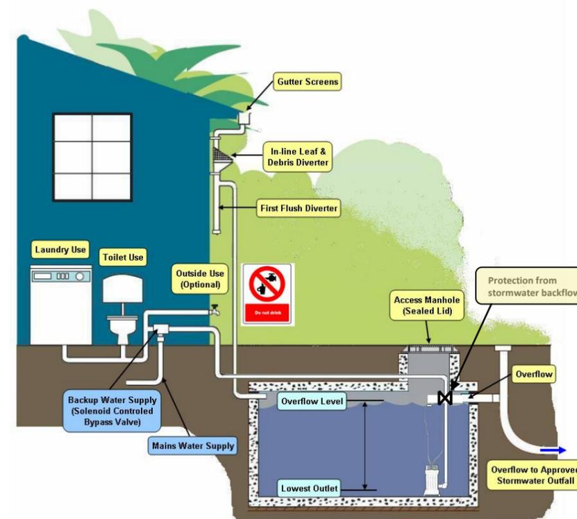
Figure 3: Rain Tank below ground - typical components
