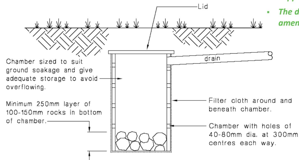
Figure 1: Typical Chamber Soak-pit
