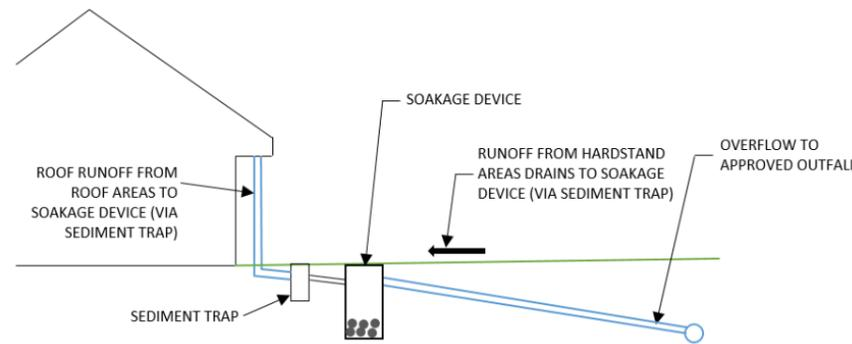
Figure 3: Schematic showing typical arrangement for soakage reduced
