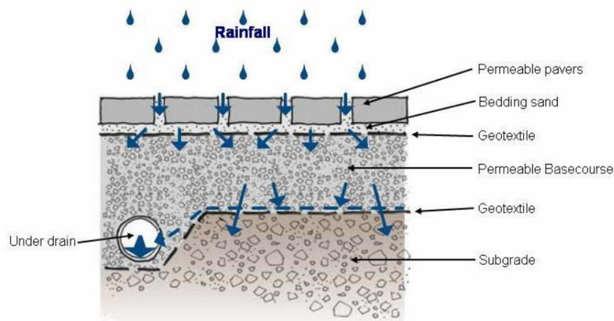
Figure 1: Typical layers in permeable pavement
