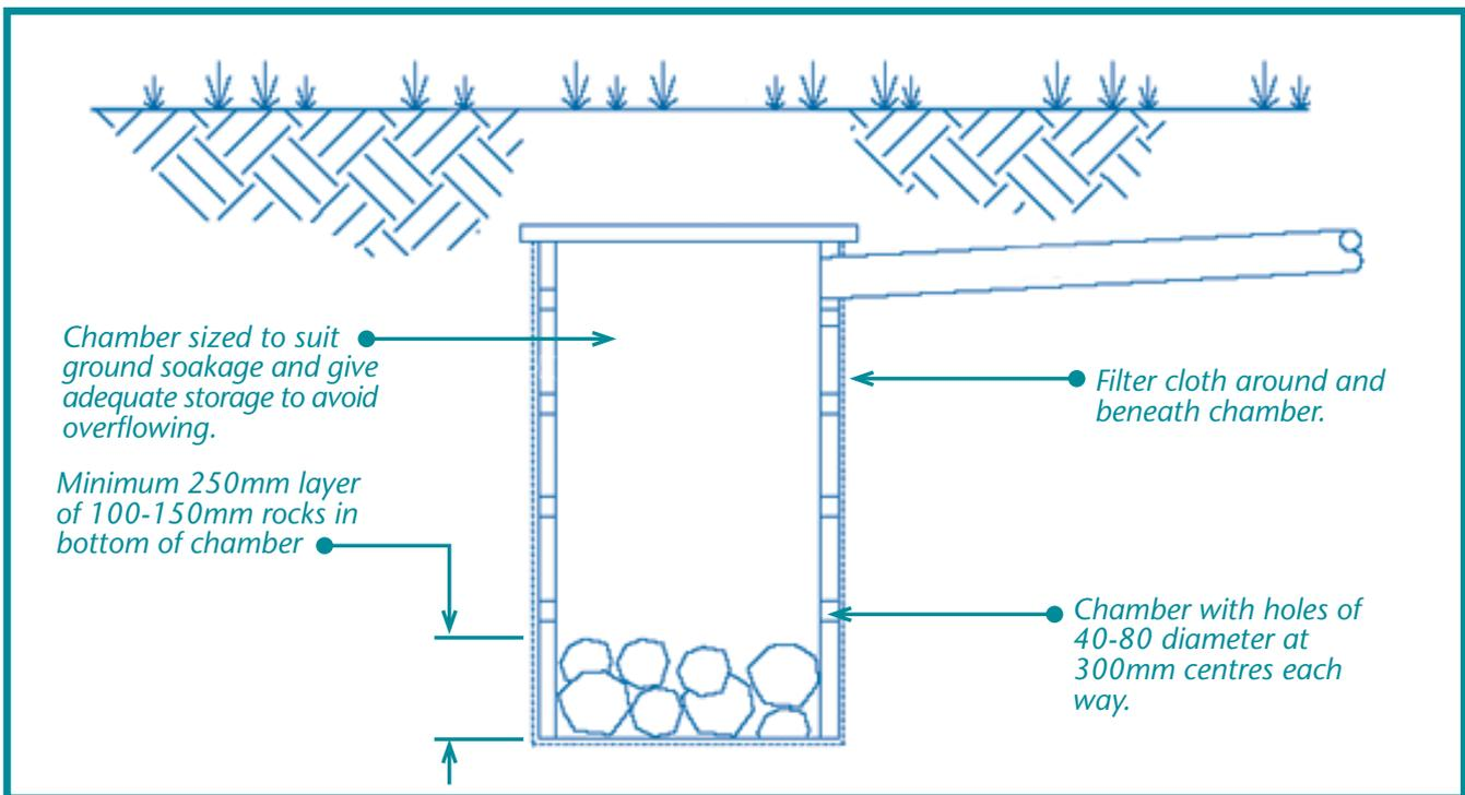
Figure 1 - TYPICAL CHAMBER SOAKPIT
