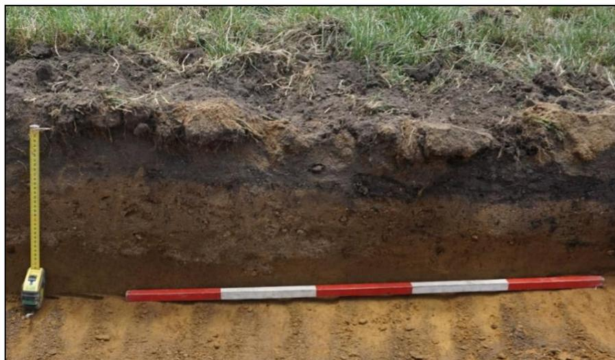
Figure 2: Profile of Geotechnical test pit 4 (S14/318). Note the anthropic sand and gravel between the topsoil and B-horizon.
